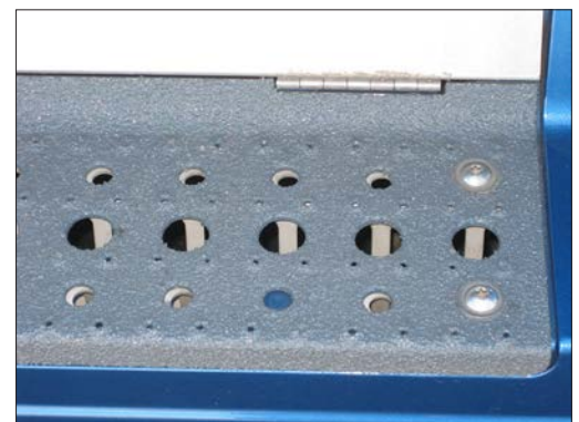
Direct Gritting on OEM step Maintains pass-through and functionality
